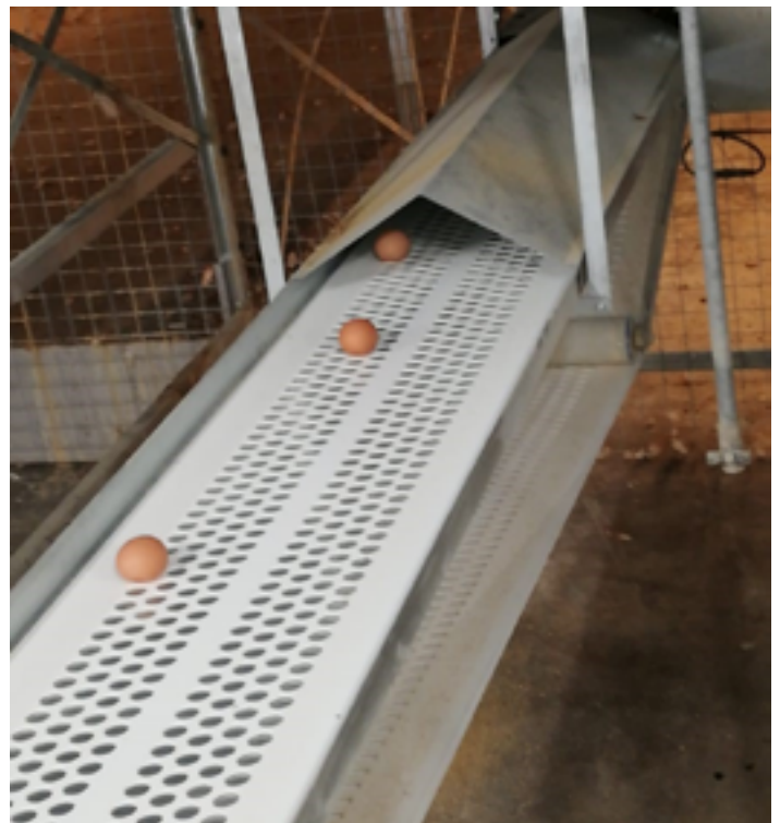
Figure 2 - The automatic nest box system with egg collection (photo courtesy of Deon Venter- Afrivet)
